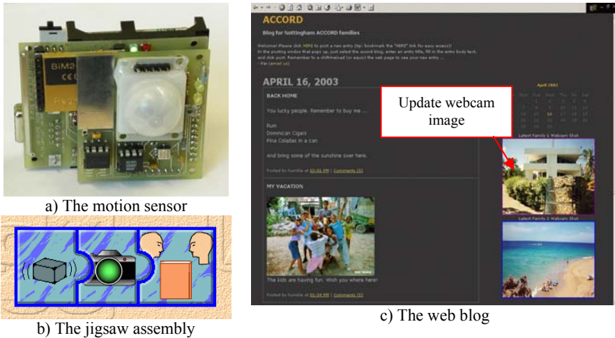
Fig. 13. Combining a Lightweight Sensor, a Device, and an Application to Monitor a Space
